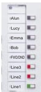
These eight keys can be assigned to PBX functions such as Call Forward(FWD) / Do Not Disturb (DND), and Conference. Each has a dual-colour LED that shows the line status, extension status, on/off, and other information.
