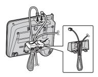
2 Connect the telephone line cord. Drive the screws (not supplied) into the wall. Mount the unit, and then slide it down. Connect the AC adaptor to power outlet (page 8).
